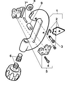
\*Three Roll Housing Screws (Ref. No. 4) used in place of Roll Pins.
